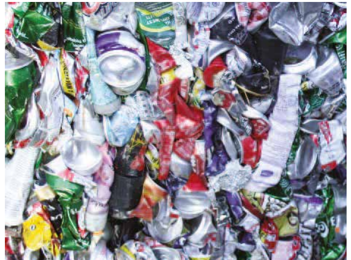
High aerosol content lead to this load being rejected.
