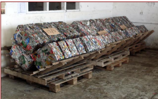
Bales are stacked for at least 3 days to allow moisture to drain.
